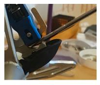
In this locked position, there will be no triggering nor manual opening and a screwdriver is required to get out of it=> Always test manual opening to ensure proper operation before going on the water.
