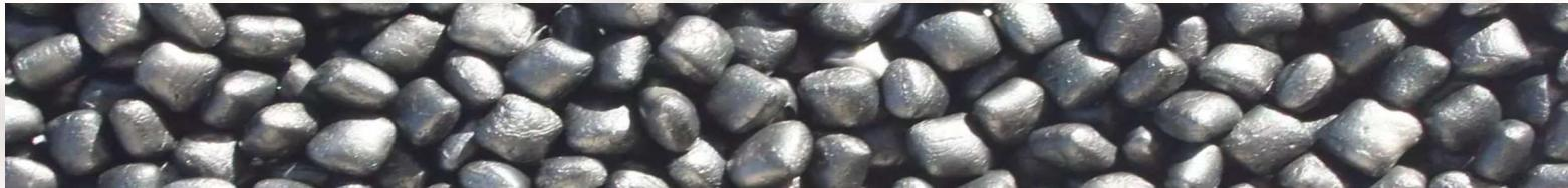
**EPP** is a polypropylene foam consisting of expanded, predominantly closed-cell foam particles.
