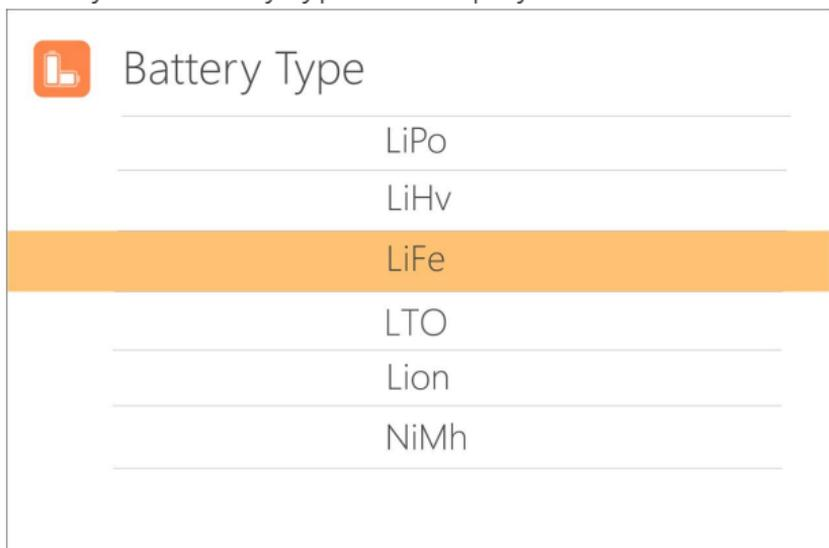
The charger supports Lipo, LiHV, LiFe, Lion, NiMh, PB, 6 kinds of batteries, after choosing the battery that matches the actual battery. Short press [OK] and [CH/Exit] to take effect, and return to the previous interface.
