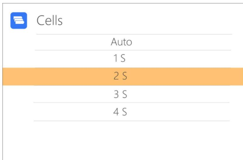
Scroll [Scroll Wheel] to adjust the value. When set to "Auto", the charger will automatically identify the number of cells connected to the battery according to the battery voltage connected to the output port. Short press [OK] and [CH/Exit] to take effect and return to the previous interface.
