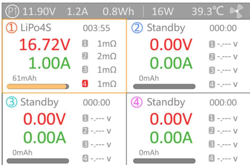
**1 1mΩ:** Internal resistance of the first battery
