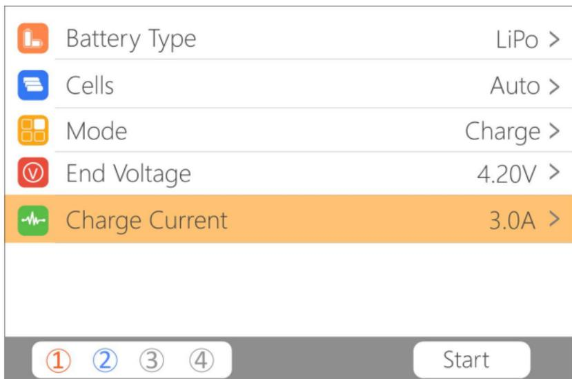
Move the cursor to "Battery Type" and press [OK] to modify the battery type, the display is as follows:
