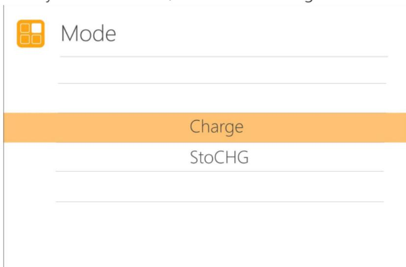
**Lipo**, **LiHV**, **LiFe**, and **Lion** batteries can be charged and stored. **NiMh**, battery and **PB** battery can choose to charge. Short press [OK] and [CH/Exit] to take effect, and return to the previous interface.
