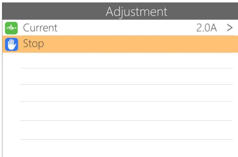
To end the charging and discharging work, short press [OK], move the cursor to [Stop], short press [OK], stop working and return to the main interface.
