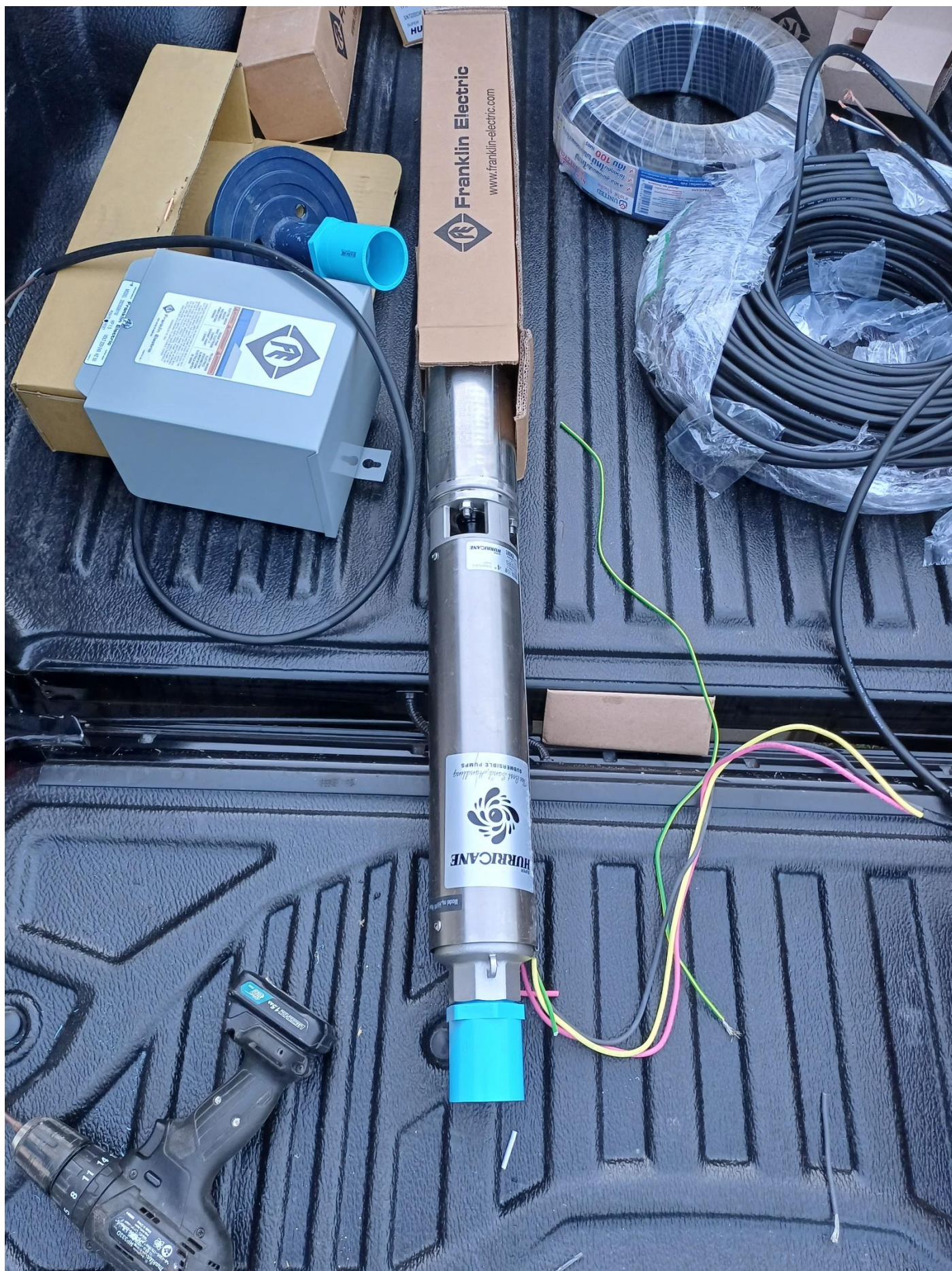
De RVS dompelpomp / The stainless steel submersible pump / Die Edelstahl Tauchpumpe – Ø 4" | 100 mm
