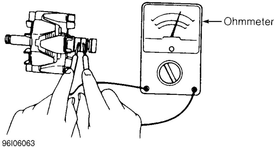
**Fig. 9: Checking Rotor Resistance**
