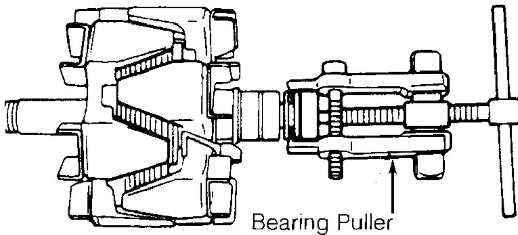
**Fig. 11: Removing Rear Bearing**
