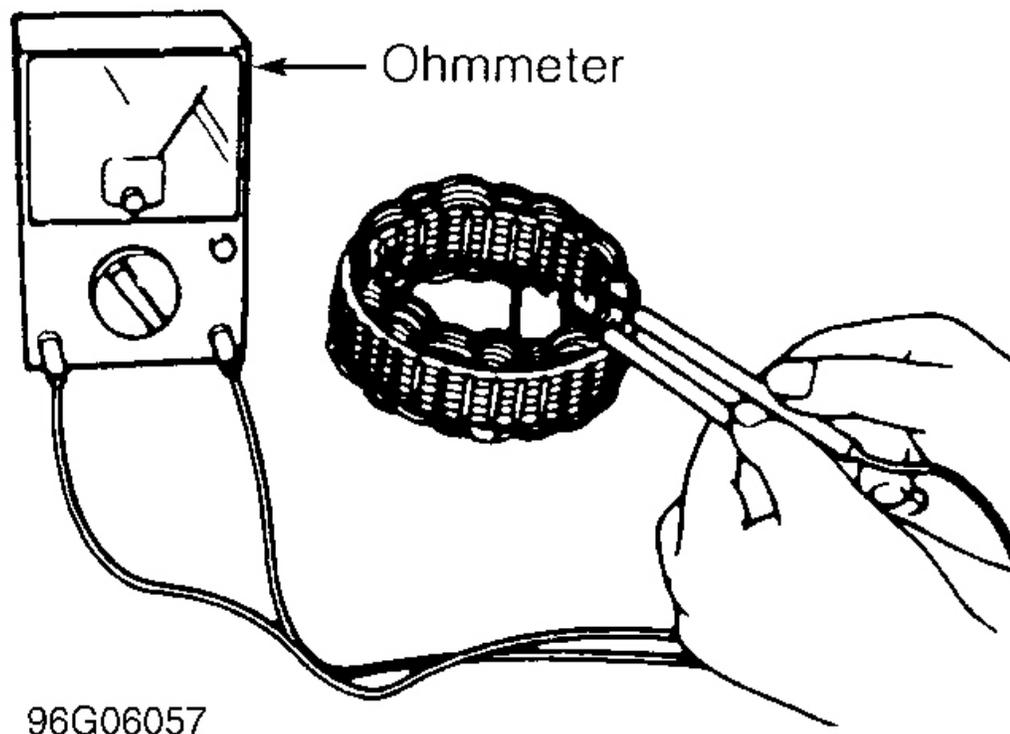
**Fig. 6: Checking Stator Winding Continuity**
