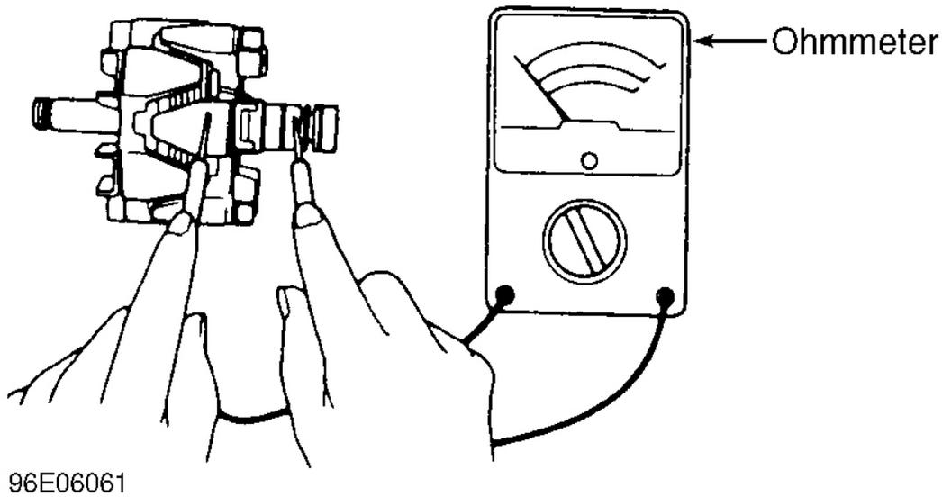
**Fig. 8: Checking Rotor For Shorts**
