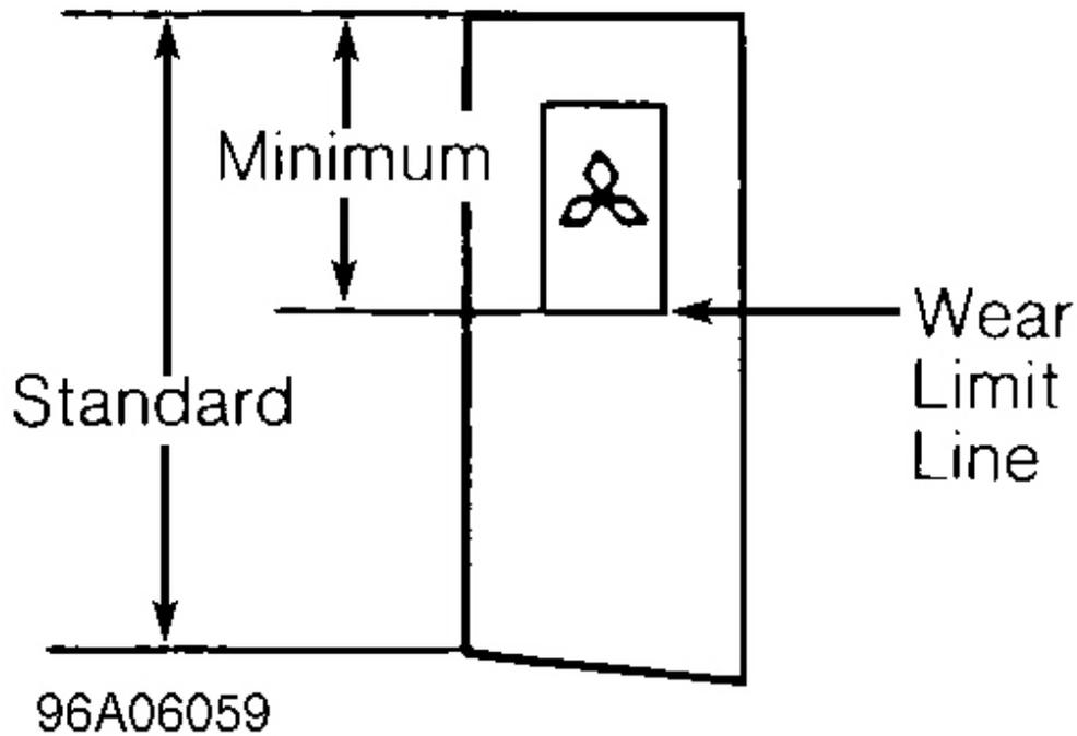
**Fig. 7: Measuring Brush Wear**
