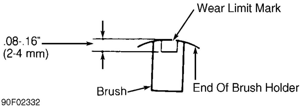
**Fig. 16: Measuring Installed Depth Of Brush**
