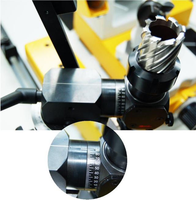
Turn the core drill support to 90° (see picture above).
