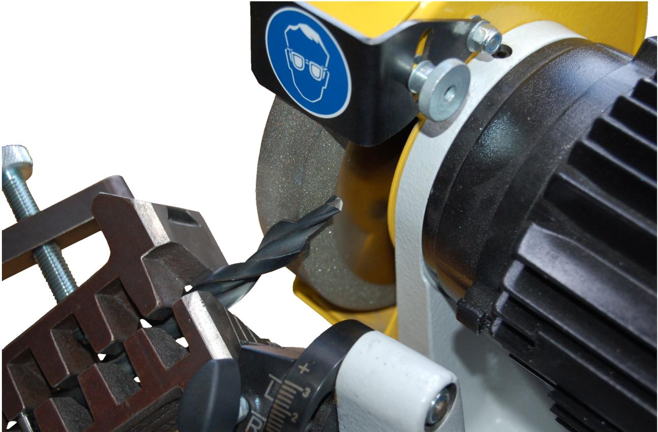
Grinding of the 1. step (tip): **Alignment and sharpening as for right hand drills** (see picture below).
