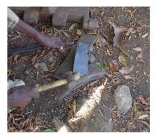
FIGURE 17 Demonstration of usage of blacksmithing tools: a metal rod held over an anvil with a tong and struck with a hammer, Aţeyä (B. Kribus/V. Krebs)
