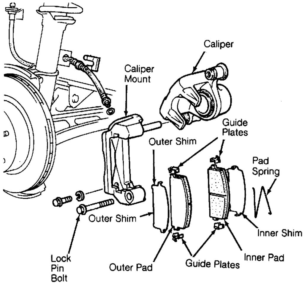
**Fig. 11: View of RX7 Single-Piston Caliper Front Brake Assembly**
