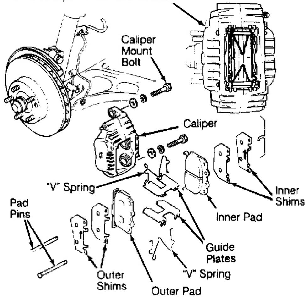
**Fig. 6: Front Disc Brake Assembly (RX7 with 4-Piston Caliper)**
