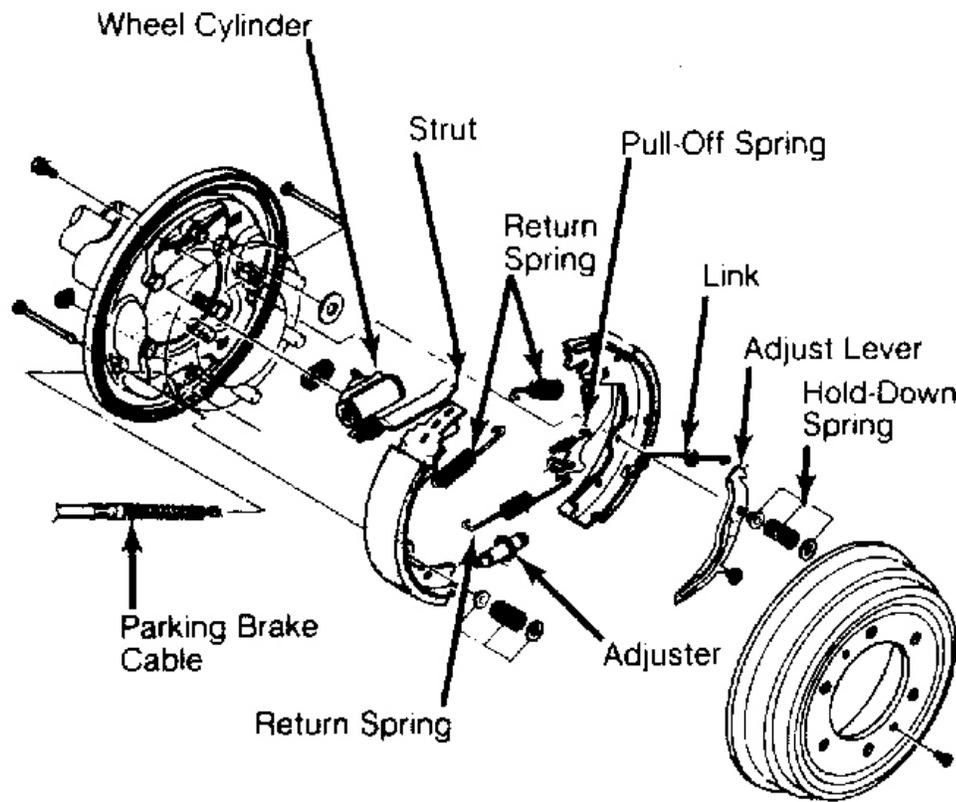
**Fig. 17: Rear Drum Brake Assembly (B2600i 4WD & MPV)**
