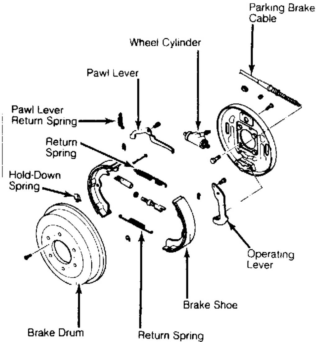
**Fig. 16: Rear Drum Brake Assembly (B2200 & B2600i 2WD)**
