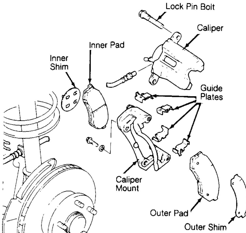
**Fig. 12: View of Front Disc Brake Assembly 929**
