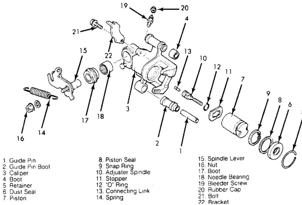
**Fig. 23: Rear Caliper Assembly (Miata, Protege & 323)**
