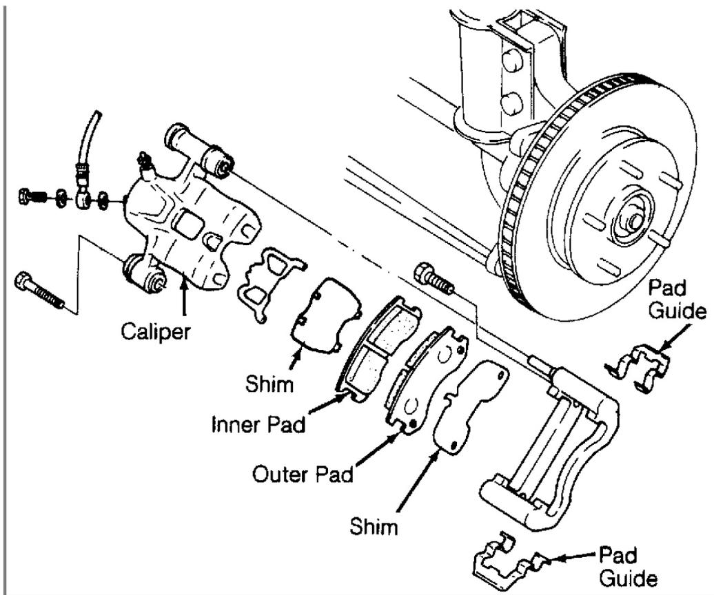
**Fig. 10: View of Front Brake Disc Assembly MX-6 & 626.**
