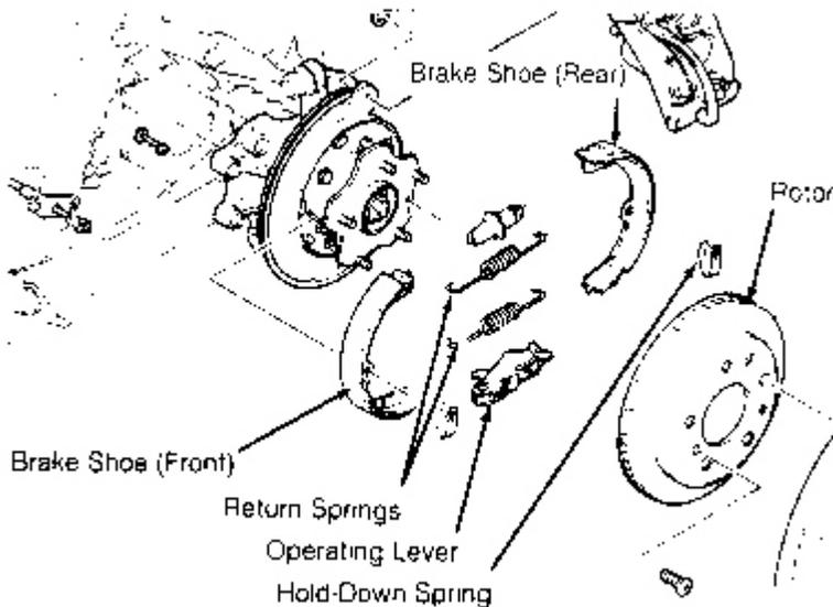
**Fig. 21: Exploded View of Parking Brake Assembly (929)**
