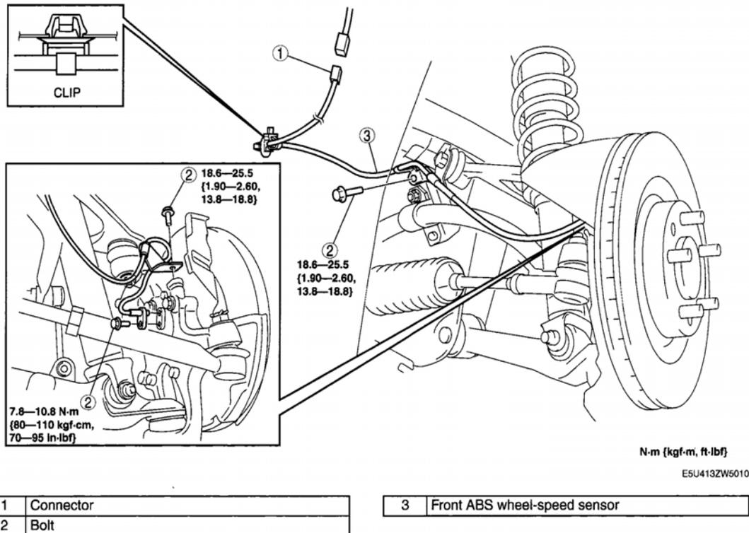
**Fig. 11: Identifying Front ABS Wheel-Speed Sensor (With Torque Specifications)**
