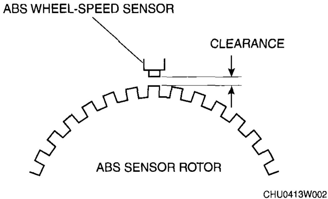
**Fig. 15: Inspecting ABS Sensor-To-Rotor Clearance**
