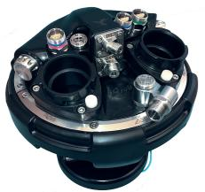
Shearwater SOLO/OBOE board is built in the hermetic compartment inside the Head. It serves ppO2 readings from three O2-sensors, setpoint maintaining, solenoid firing, HUD control, CO2 reading, HP reading on Oxygen and Diluent. If any fault on the controller or its cable is cut, the unit will still carry on working and maintain the ppO<sub>2</sub> up to surfacing.
