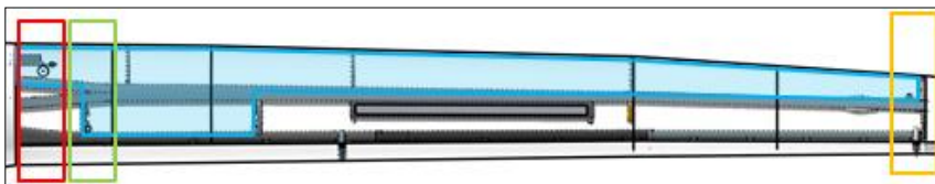
Figure 7.8-2: Main wing tanks (blue)
